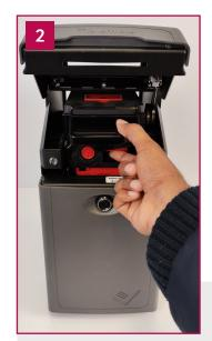
Lift the red head release latch on the front of the unit, then slide the head forward to remove it from the LiveSafe chassis.
