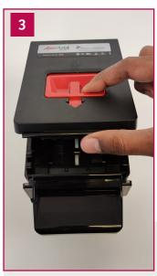
Pull the red cover release latch forward to unlatch the note path, then pull upwards to open the note path.
