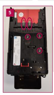
Flip the head and carefully wipe the surfaces of the sensor lenses highlighted below.
