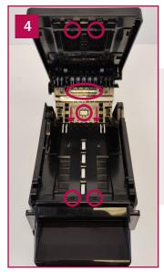
Clean the note path and sensors with a clean Tellermate microfibre cloth. Do not use lubricants or cleaning products.
