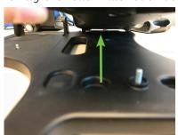
Insert the black button screw and twist clockwise until secure.
