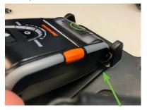
Ensure mounted screw is aligned with printer.
