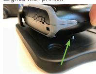
Twist clockwise to tighten the button screw until secure.
