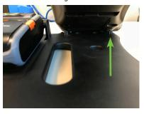
Ensure the back tabs fit into place, then lay the Tellermate Touch down.
